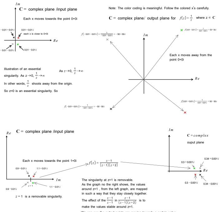
We can see the output points are moving towards a certain value. Thus the singualirty that arises from the presence of z-1 can be removed simply by redefining the value of the function to be equal to the limit that f(z) approaches as  $z \rightarrow 1$ .
